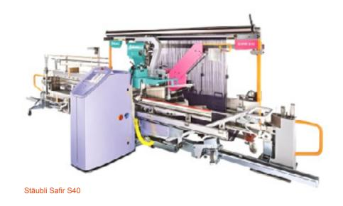
While drawing in is being done at the first station, the next warp sheet is being prepared at the second station, so that the drawing-in machine is constantly in productive use. The modular design of the system allows the mill to gradually expand its drawing-in capacity as changing needs dictate. All these advantages make the SAFIR S40 the perfect solution of automatic drawing in of Denim fabrics.
