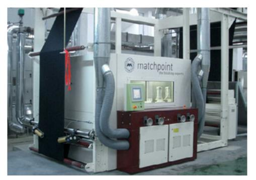
Using the diamondpeach technology at diamondTec sueding machine © Photo Matchpoint Textilmaschinenbau
