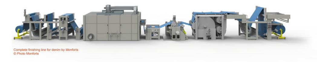
Finishing on a sanforizing line gives the fabric a more stable structure, a silky shine, a smooth hand and minimum residual shrinkage values. BRÜCKNER offers single or double sanforizing lines and combinations with felt calenders depending on the product and the customer's requirements.
