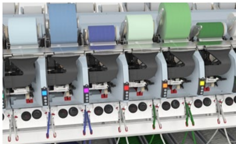
The Autocoro 11 rotor spinning station equipped with the new Duo Sliver Feeding concept. © 2026 Saurer
