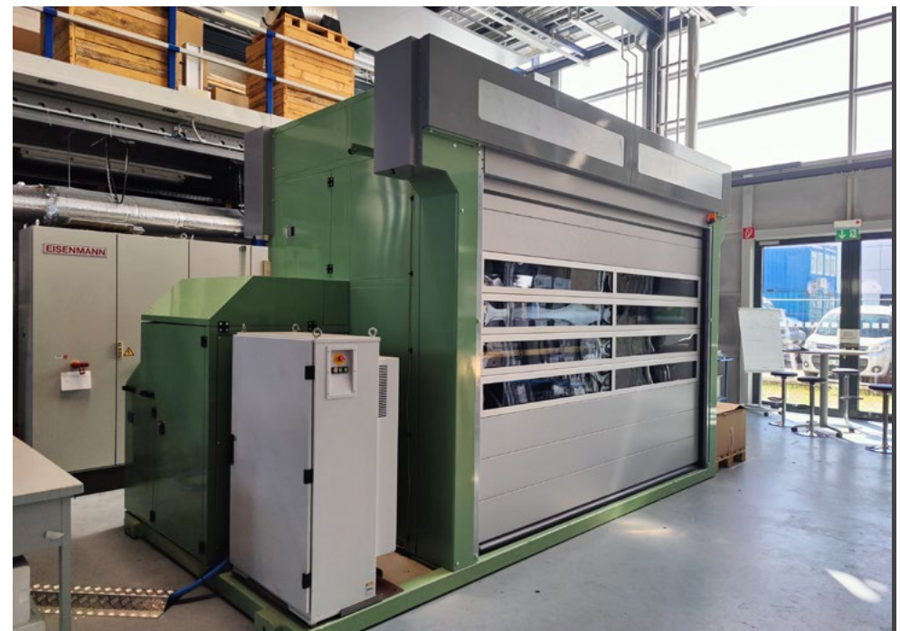
Fig. 1: Fully encapsulated Dornier A1 air-jet loom at ITA, RWTH Aachen (Source & Copyright: ITA)
