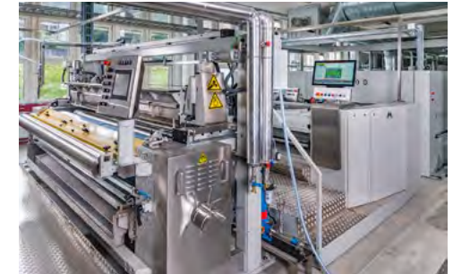
MontexCoat unit installed in front of a MONTEX stenter © 2026 Monforts
