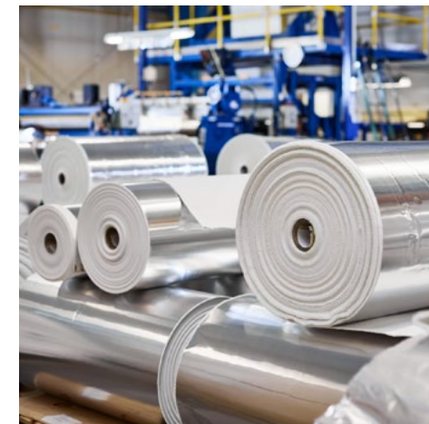
Manufacturing process: Laminating, glass fleece with aluminum lamination © 2026 Photo: ASGLAWO group, Jan Felber
