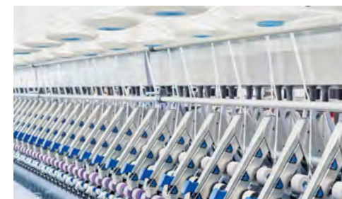
The ZI 451 worsted compact-spinning machine processes long staple fibres, such as wool © 2023 Saurer
