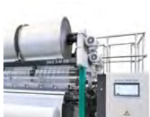
High-performance warp knitting machine with energy-efficient direct drive © 2023 KARL MAYER
