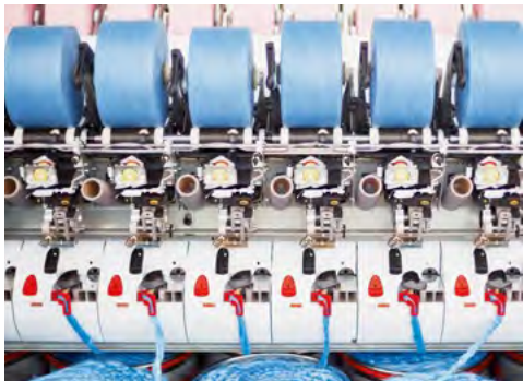
BD 8 semi-automatic rotor-spinning machine for producing yarns from recycled fibres © 2023 Saurer
