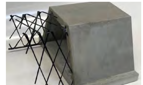
Embedded textile mesh girder © ITM/TU Dresden
