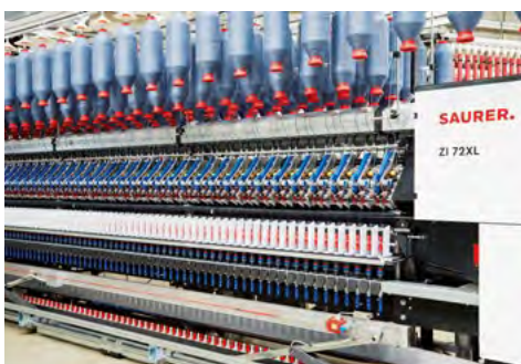
ZI 72XL compact-spinning machine processes recycled yarn © 2023 Saurer
