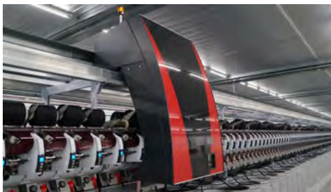
Autocoro 11 rotor-spinning machine for producing yarns from recycled fibres © 2023 Saurer
