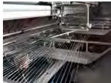
Weft Carrier on a warp knitting machine with weft insertion © 2023 KARL MAYER
