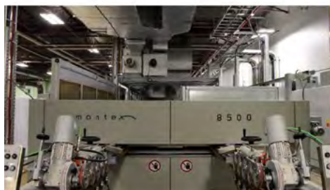
Canada's Albarrie is now benefiting from one of the first Monforts Montex stenter installations equipped with the full range of MonforClean heat recovery and exhaust air purification technologies. © 2023 Monforts
