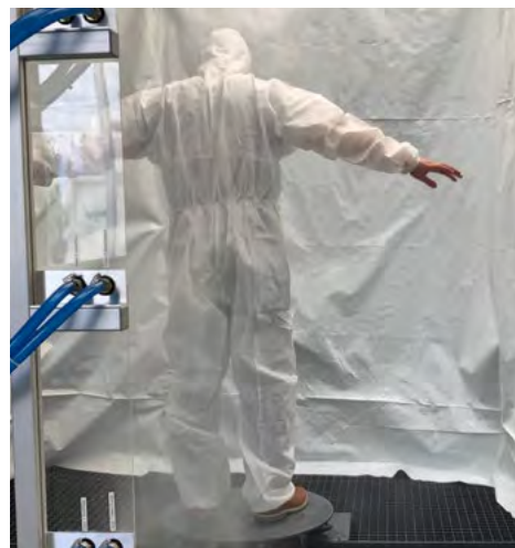
A chemical protective suit protects the person wearing it from chemicals in gaseous, liquid and / or solid state. They are classified into 6 types with different protection levels from gas-tight to restricted liquid-tight © Hohenstein
