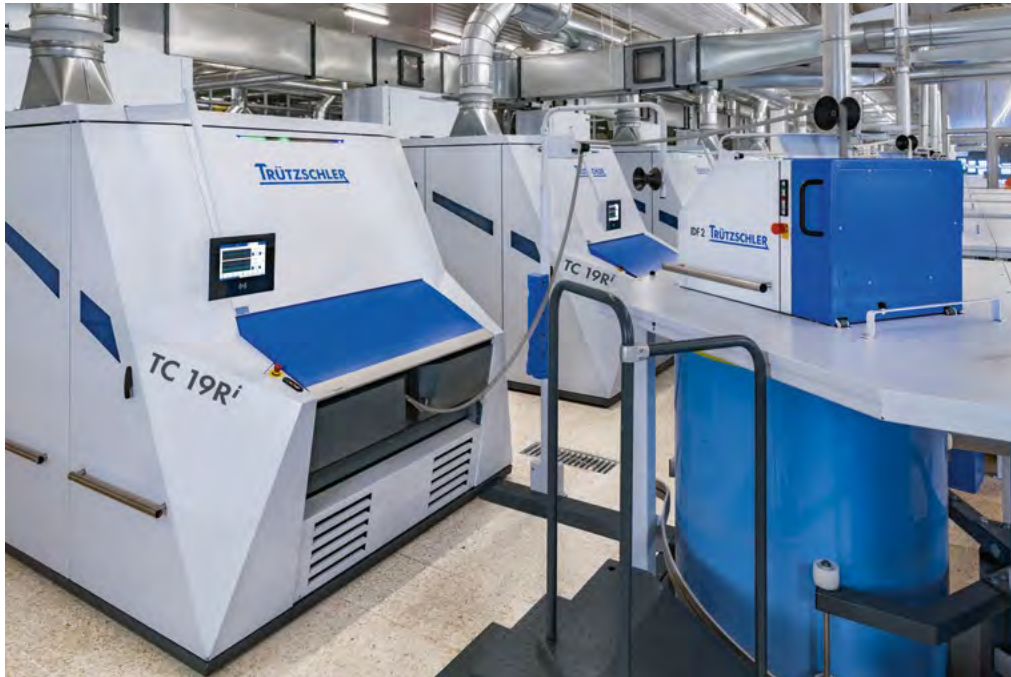
Trützschler offers proven solutions for textile recycling – such as the intelligent card TC 19Ri for Recycling © 2023 Truetzschler
