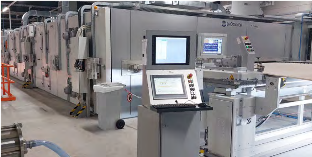
Electrically heated DUO-THERM oven for nonwoven finishing © 2023 Brückner
