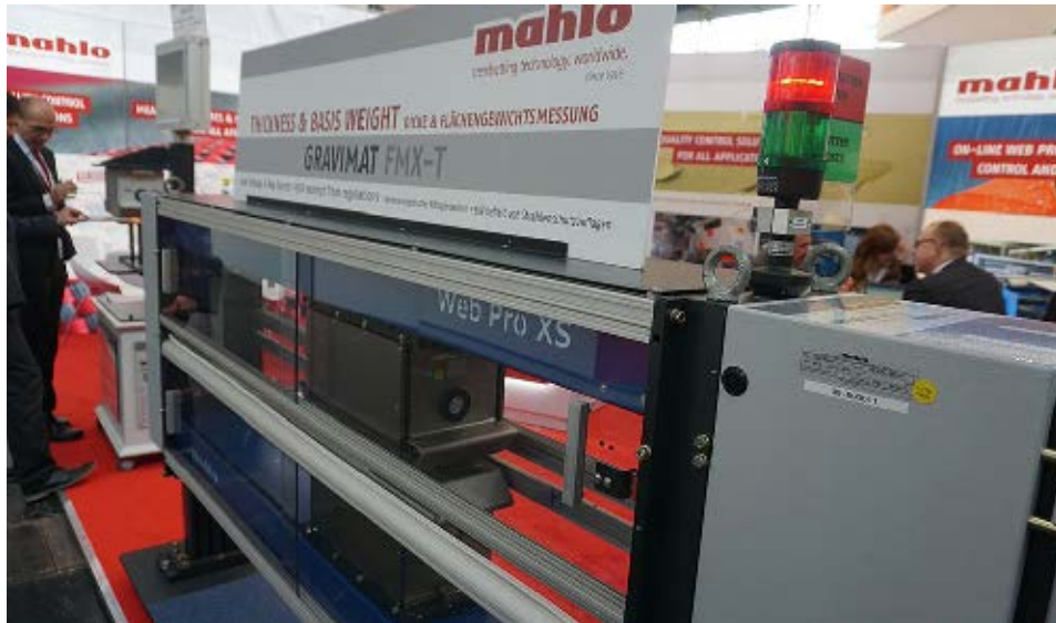
Mahlo Compact O-frame Webpro XS with an X-ray basis weight sensor Gravimat FMX-T (c) 2017 Mahlo
