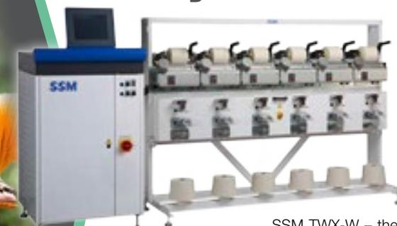
SSM TWX-W – the cost-efficient precision package winder for dye-packages and rewinding applications. For the flexible processing of staple yarns and textured filament yarns.
