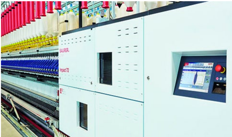
ZinserImpact 72 compact spinning machine (c) 2017 Saurer
