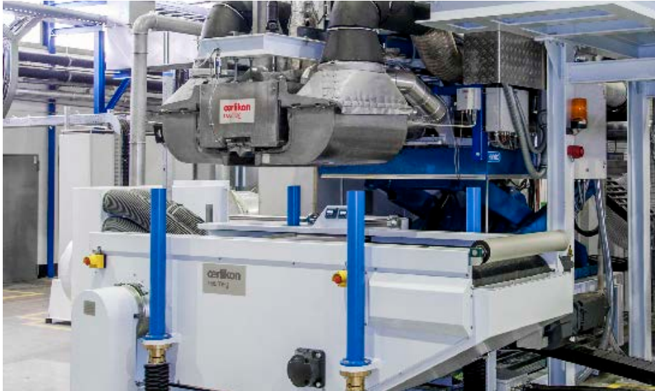
Oerlikon Neumag's multifunctional forming table for meltblown systems with a considerably reduced footprint and a shortened wire length that reduce maintenance costs. (c) 2017 Oerlikon
