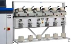
SSM TWX-W – the cost-efficient precision package winder for dye-packages and rewinding applications. For the flexible processing of staple yarns and textured filament yarns.
