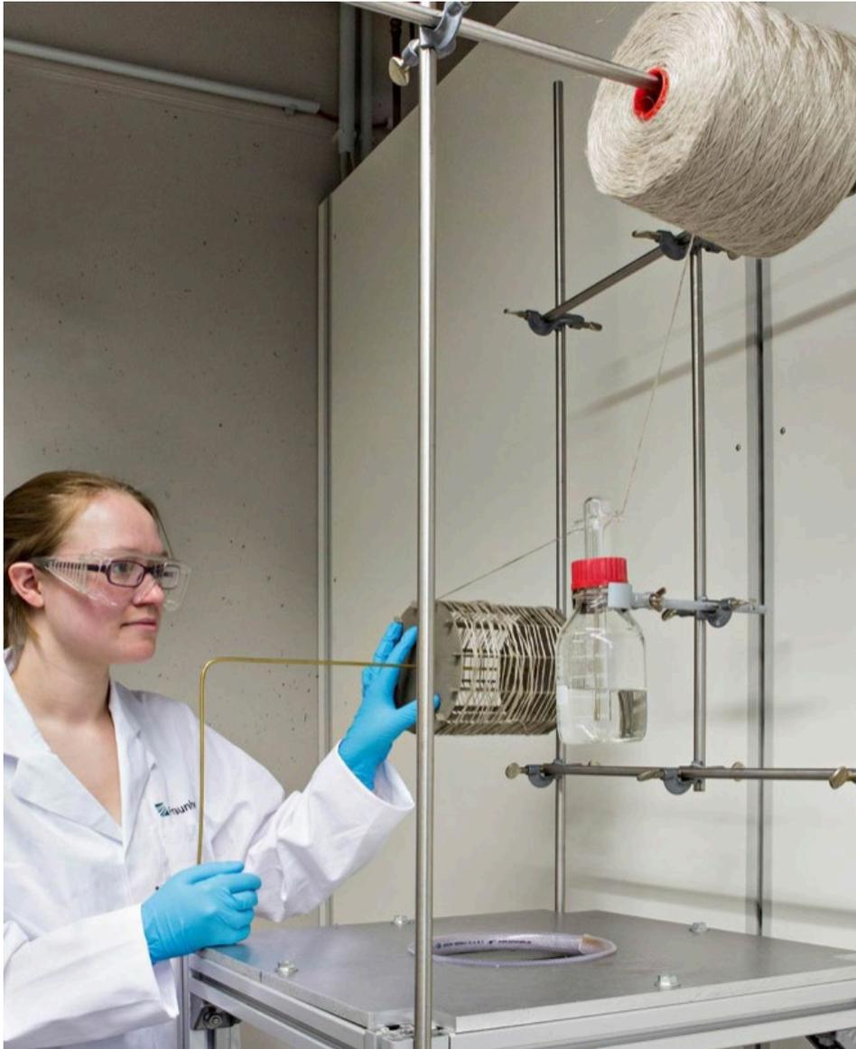
Configuración experimental del pre tratamiento de fibra (c) 2017 Fraunhofer Institute for Structural Durability and System Reliability LBF
