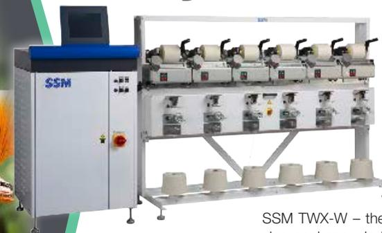
SSM TWX-W – the cost-efficient precision package winder for dye-packages and rewinding applications. For the flexible processing of staple yarns and textured filament yarns.
